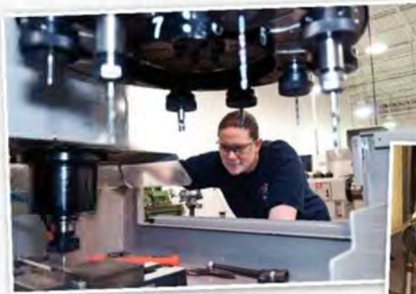
Penn College's automated manufacturing program features a Haas Technical Education Center with computer numerical control (CNC) machine tools provided by industry leader, Haas Automation Inc. Here, student Britni M. Fennell works on a Haas vertical machining center.
